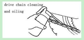
A dirty drive chain may not only accelerate the chain wear, but also damage the sprocket. Therefore after cleaning it with clean deterging. Smear the drive chain with special chain oil or engine oil.
